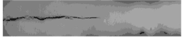
Fig. 5. Segmentation of a welding radiograph [47]
