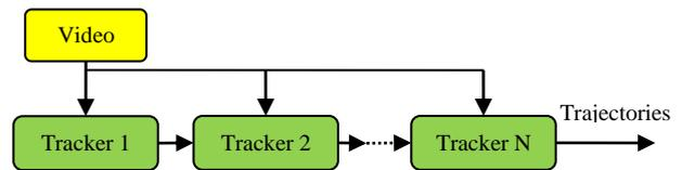
Fig.4: Sequential integration of tracking estimates in a cascade architecture.
