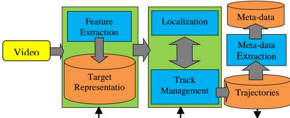
Fig.1: The video-tracking pipeline.
