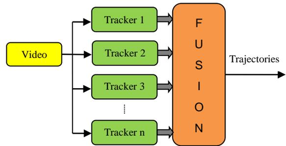
Fig.3: Fusion of independent estimates from parallel trackers.
