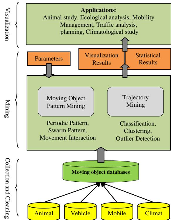
Fig.5: Architecture of a tracker system for motion mining.
